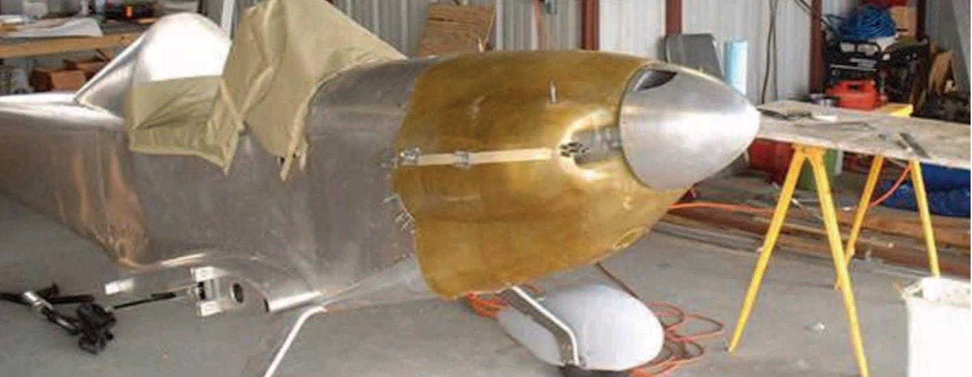
The cowl is cut along the side, separated, and a 3/4-inch lip added to the inside of the lower half of the cowl to provide an area for the top cowl to attach to. Tinnerman nuts were added to this lip every 3 1/2 inches to fasten the two halves together. Two more plies of fiberglass were added to the inside of the cowling. The completed assembly was sanded to the desired finish.
