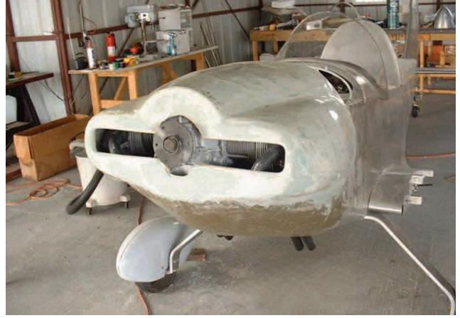
Above, left: Cowl ready for duct tape to be applied, and Bondo body filler to be applied over that. The cowl is then sanded to desired finish, and 2" clear packaging tape is applied over the cowl. That's then waxed and fiberglass applied.
